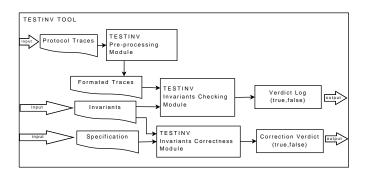
Figure 2. Basic architecture of the TestInv tool.
