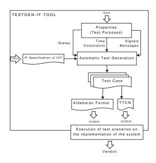
Figure 1. Basic architecture of the TestGen-IF tool.
